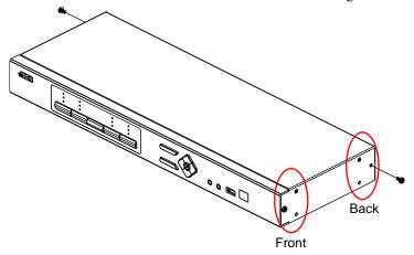
**Note:** You can remove the screws on the front side panels or the back side panels. The succeeding diagrams show the rack mounting steps for the back panel.
